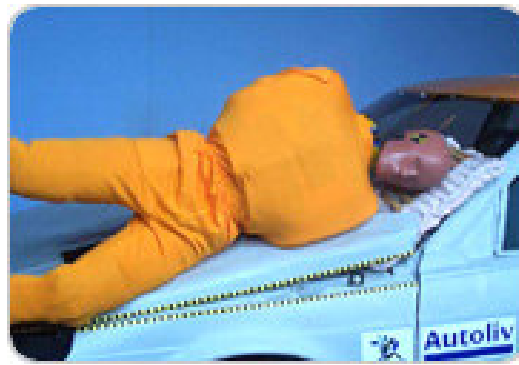
Figure 23. Example of an airbag used to prevent hard contact between the head and the A-pillar (Source: www. Autoliv.com )
